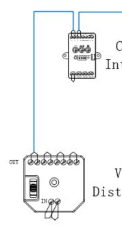
Connected to the video distributor 'in' port: all the branches of the video distributor will received the video.
