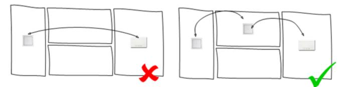
**3.** The devices should not be installed directly next to large metal surfaces.
