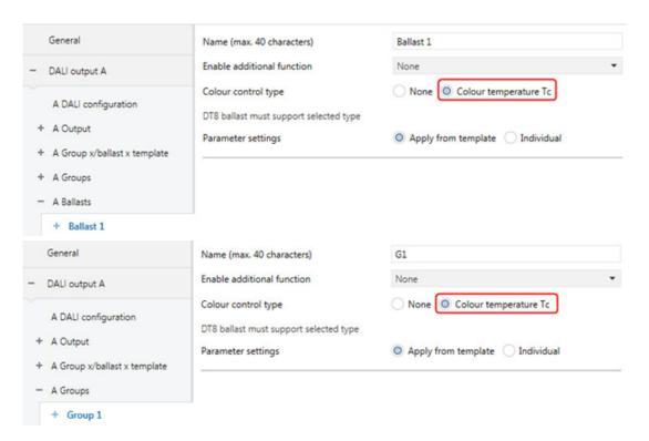
To complete the basic conditions, it is important to determine the minimum and maximum color temperatures of the group or ballast.
